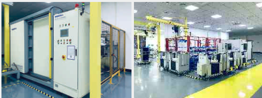
Vacuum tank helium leak detection system
